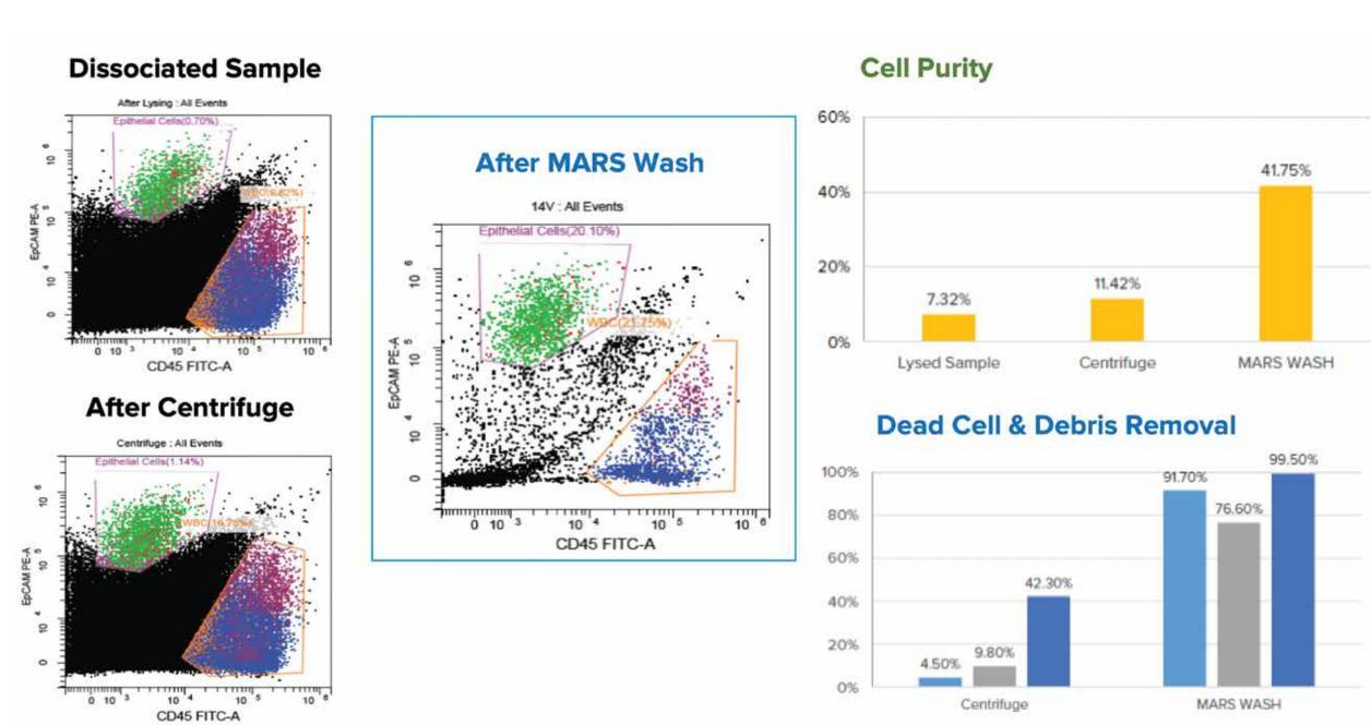
Tumor biopsy dissociated cell suspension was processed by centrifuge-wash for 3x and MARS acoustic wash at 0.8mL/min one pass. MARS wash achieved higher purity and cell recovery.
