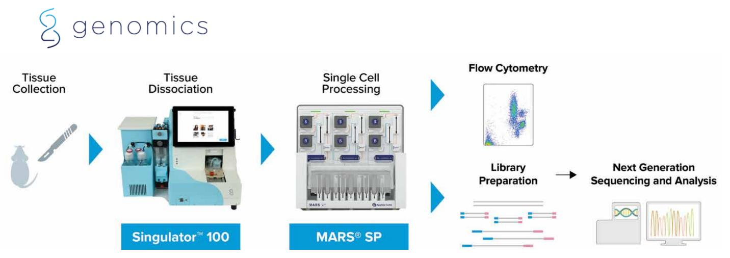
Schematic illustration of the workflow: solid tissues from various organs of the murine sample were processed on Singulator 100, and single-cell/single nuclei suspension was generated with pre-set programs. The cell/nuclei suspension was then processed on MARS acoustic module with a "Wash" program to separate cells/nuclei from debris. "washed" cells/nuclei will be ready for flow cytometer analysis or downstream single-cell genomics analysis.
