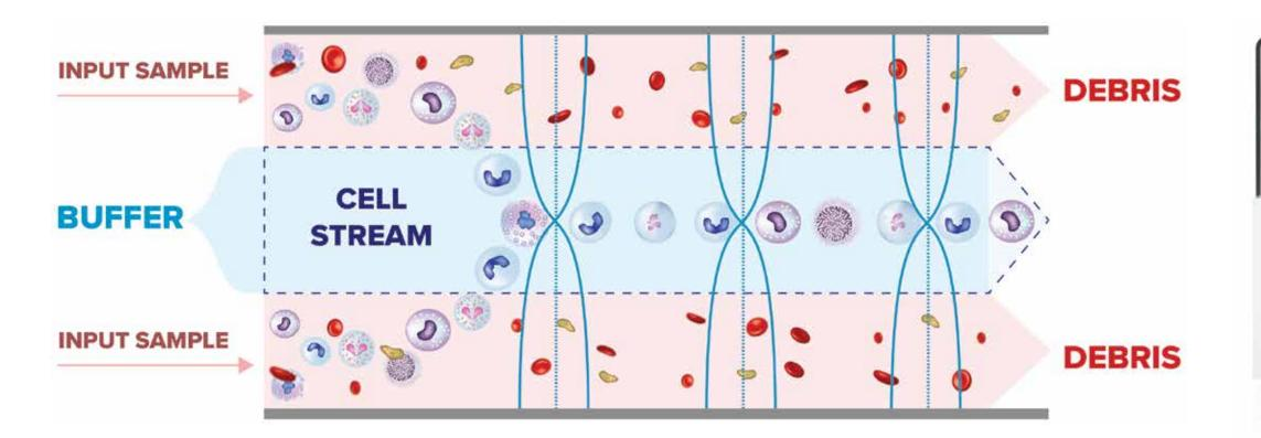
Schematic explanation of MARS Acoustic Cell Separation/Washing process: cell suspension that contains live cells, dead cells and cellular debris passes through a microfluidic channel in a laminar flow with the "wash buffer". When the acoustic field is turned on live cells will move to the "wash buffer" from the original suspension but dead cells and debris will exit the channel before they move to the "wash buffer". The flow rate of the sample and "wash buffer" are both 0.8mL/min.
